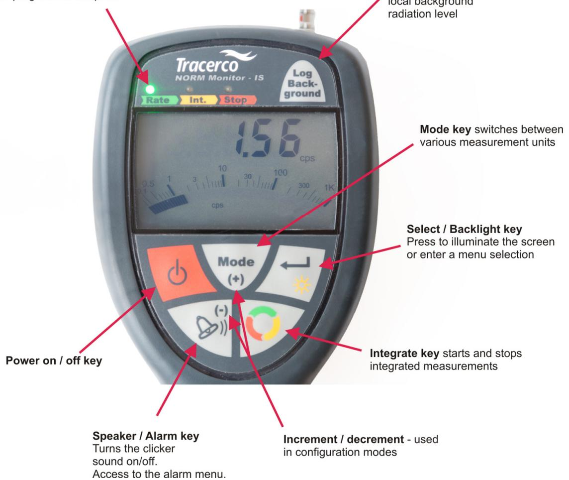
Figure 3 - Tracerco *NORM Monitor-IS* – key definitions
